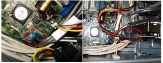
14. Connect the ODD data cable and power-cable to the rear of ODD.
